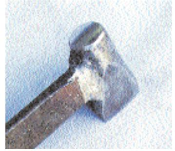
Any struck tool will need cleanup and maintenance on a regular basis. A driving hammer with its edges and the off center blows on a clinch cutter will cause minor mushrooming and then small chips to break loose. Be sure to dome the struck end of your tools and put a good chamfer on the edge.
