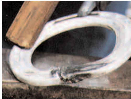
8. Don't forge or hammer the shoe until it has cooled. Burn mark from handle indicates shoe is too hot at this stage
