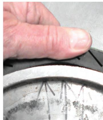
ABOVE: OPERATION OF WHEEL WITHOUT BELT CAN CAUSE DAMAGE TO RUBBER SURFACE AND MAY EVEN ALLOW SEPARATION OF RUBBER FROM METAL HUB
