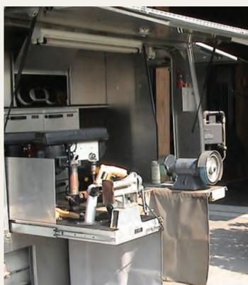
FARRIER RIG WITH GRINDER ON SLIDE-OUT
